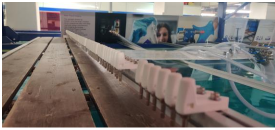
(C) 3d printed nozzles fitted to linear rail
