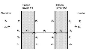
To simplify the calculations, few assumptions were made such as the glazing layer thickness is assumed to be thin as if the heat storage within the layer could be neglected. Second, the heat flow is one dimensional and perpendicular to the glazing face. Third, and as in most glass products, the gazing layers are considered opaque to infrared waves. Finally, due to the nature of glass conductivity being high, the glazing faces are assumed to be isothermal.
