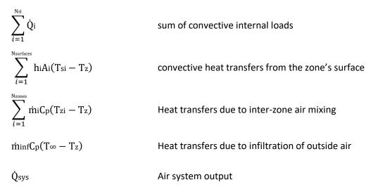
Considering the air capacitance is zero, the system can be assumed at a steady state with:
