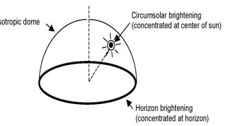
Sky clearness and brightness are the two main factors defining the proportions of these distributions, measured from the sun position and the solar measurements extracted from the selected weather files. In the simple case of no shadowing, the sky diffuse irradiance can be expressed as:
