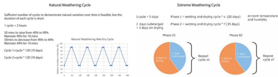
Figure 2. (a)Natural Weathering Test Design; (b)Extreme Weathering Test Design
