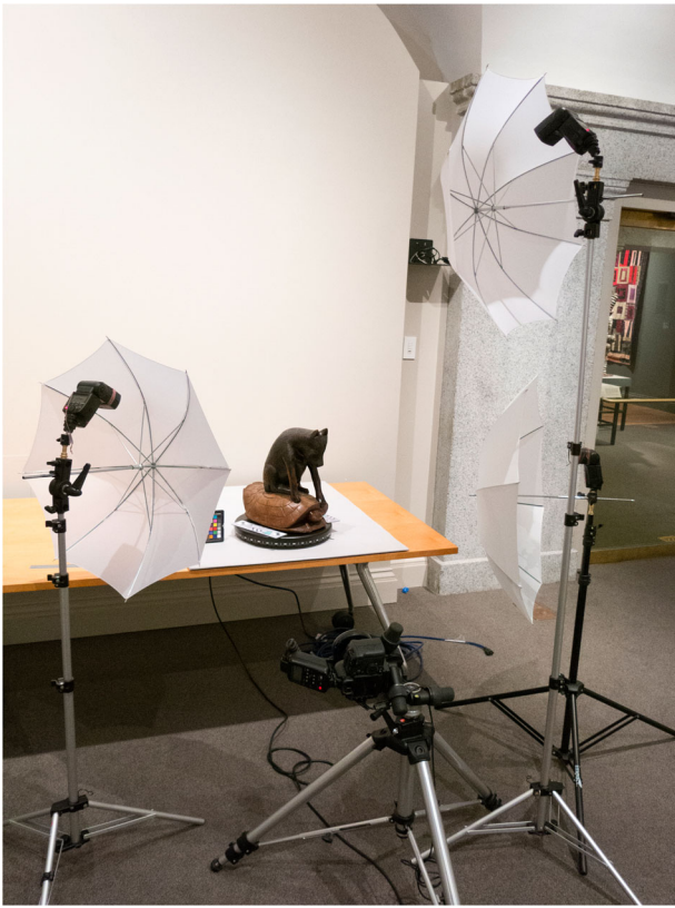
Figure 3. Imaging setup for Acquisition A that shows the object on the turntable and the positions of the lights.
