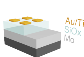
Fig. 2. Device Structure. The device studied in this paper has a metal-insulator-metal structure. The two electrical contacts are the molybdenum bottom contact and the gold top contact. A 3nm titanium buffer layer is deposited prior to the deposition of the gold, to improve the adhesion of the top contact and to serve as an oxygen getter.
