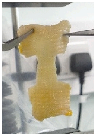
Fig. 1. A ‘dog bone’ shaped section of human posterior rectus sheath before uniaxial tensile strength testing.
