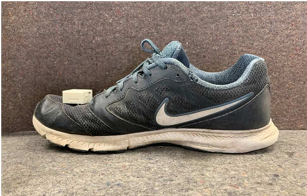
Fig. 2. Inertial Elements IMU attached to the right foot with Velcro®
