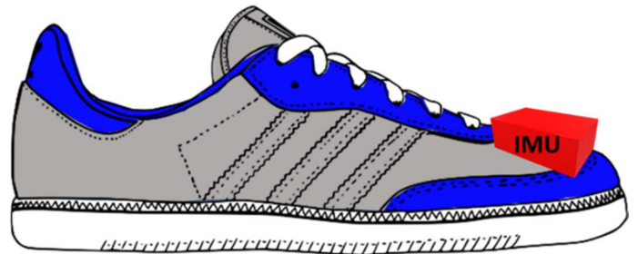
Fig. 1. IMU placement on right foot
