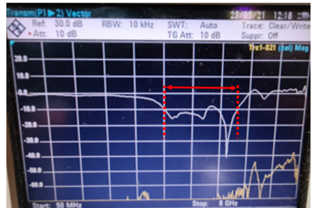
Fig. 10: Anechoic chamber measurements of antenna element return loss.
