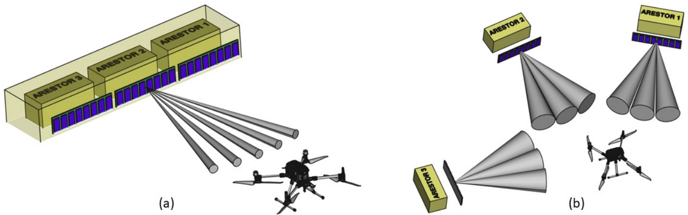
Fig. 1: Concept of modular RFSoc based monostatic array solution (a) which can be re-deployed as a distributed coherent multistatic solution (b).
