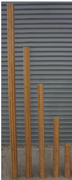
Figure 4 Specimens with different slenderness ratios
