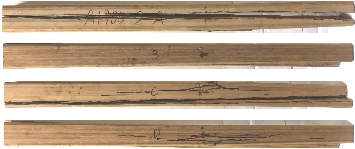
(b) Failure phenomena of A1700-2
