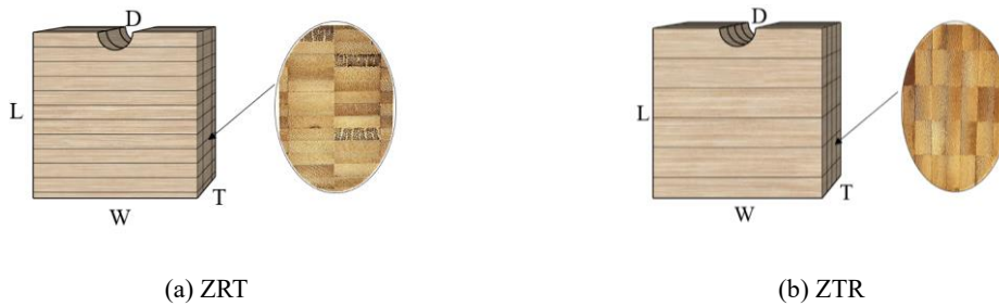
Fig. 4 Manufacturing process of the dowel-bearing strength specimen
