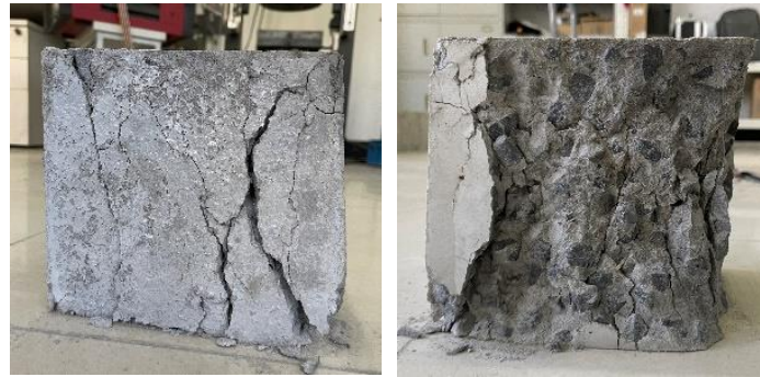
Fig.6. Failure mode of PC cubes.
