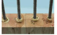
(c) Multiple rod bond failure [118]
