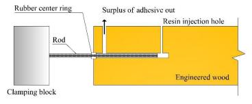
Fig.9 One of the available methods of gluing-in rods [99]
