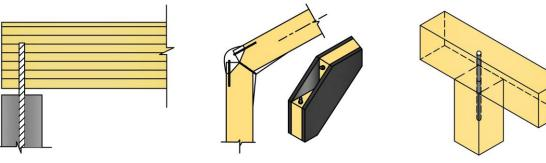
Fig.12 Examples illustrating some of the possible connection methods employing bonded-in rods
