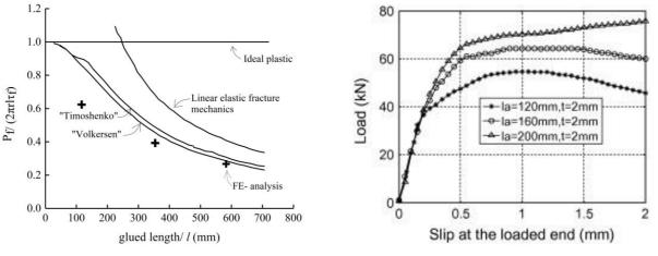
(a) Comparison of different methods (according to GIROD engineering model) [47]
