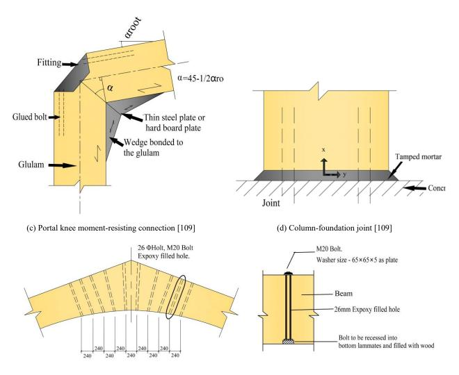
(e) Repair of a curved glulam beam with epoxied steel dowels [130]
