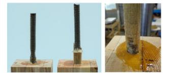
(a) Single rod yielding (left); shear block failure (middle); bond failure (right) [32]
