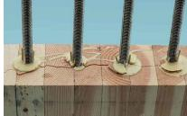
(d) Multiple rod splitting [118]Fig. 15 Specimen Sample damage images from real tests
