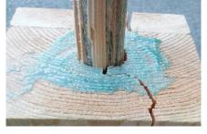
(b) Splitting of timber (single rod connection) [36]
