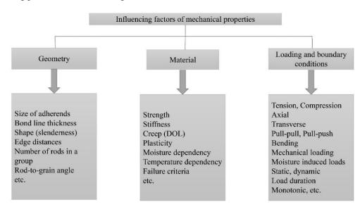
Fig.3 Influencing factors on the bond performance of glued-in connection [27]
