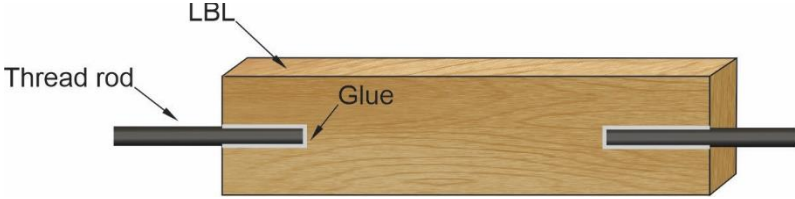
466 467 Figure 21: GIROD-LBL connection specimen (reproduced from Yan et al. [118])
