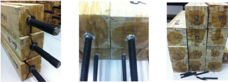
479 480 Figure 22: Typical GIROD-LBL failure modes (extracted from Zhang et al. [120])
