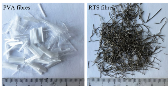
Fig. 2 Physical appearance of PVA and RTS fibres.
