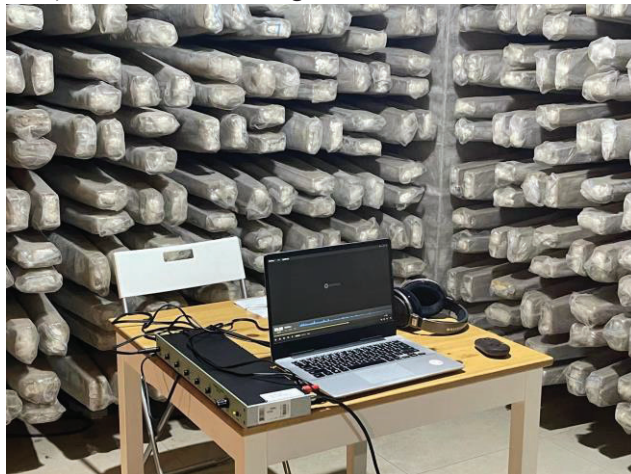
Figure 1 – Soundscape evaluation experiment in the semi-anechoic chamber
