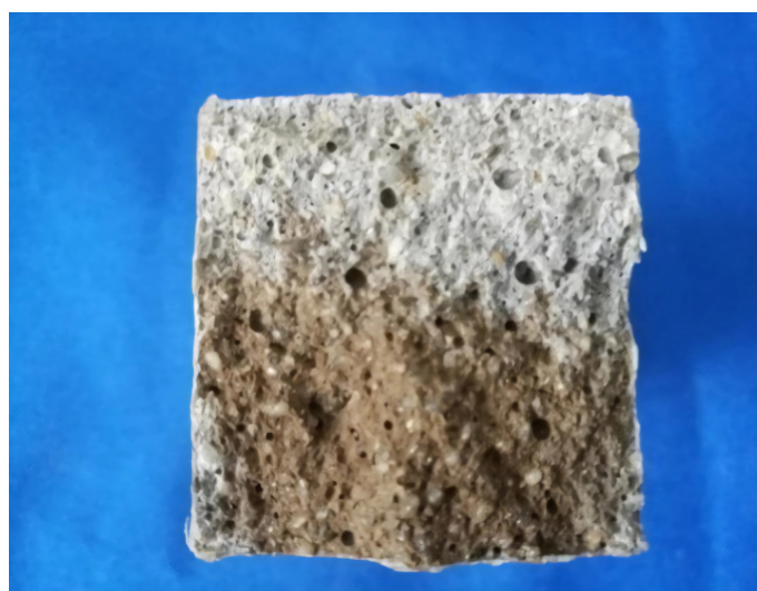
Figure 2. Chloride ion penetration area.
