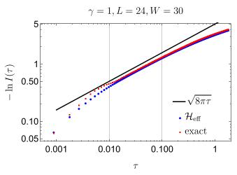
FIG. 9. Comparison between exact numerical results for evolution of I(t) with those obtained by solving Eq. (C1) averaged over 20 realizations for L = 24 and W = 30, obc.
