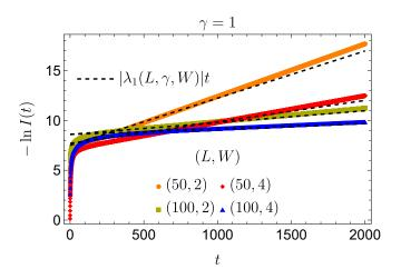
FIG. 6. Plot showing the linear growth of  $-\ln I(t)$  in region V for obc finite size systems of different lengths L and at disorder strengths W. The black dashed lines denote the expected growth of  $-\ln I(t)$  with the rate given by corresponding  $\lambda_1$  dependent on L, W, and  $\gamma$ .
