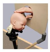
Fig. 6. Rear of the new setup showing restriction to fetal head
