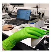
Fig. 3. Pilot study setup, with the participant using the sensor glove on the phantom fetal head
