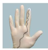
Fig. 1. The sensor glove, used to detect sutures
