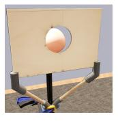
Fig. 5. Front of the new setup with a shield to fetal head
