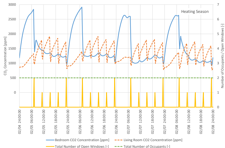
Figure 10: A 4-day section of simulation test 6 – Predicted CO 2 concentration in heating season with lockdown occupancy pattern and daytime opening of 1 to 2 windows for periods of 15 min every 4 hours.
