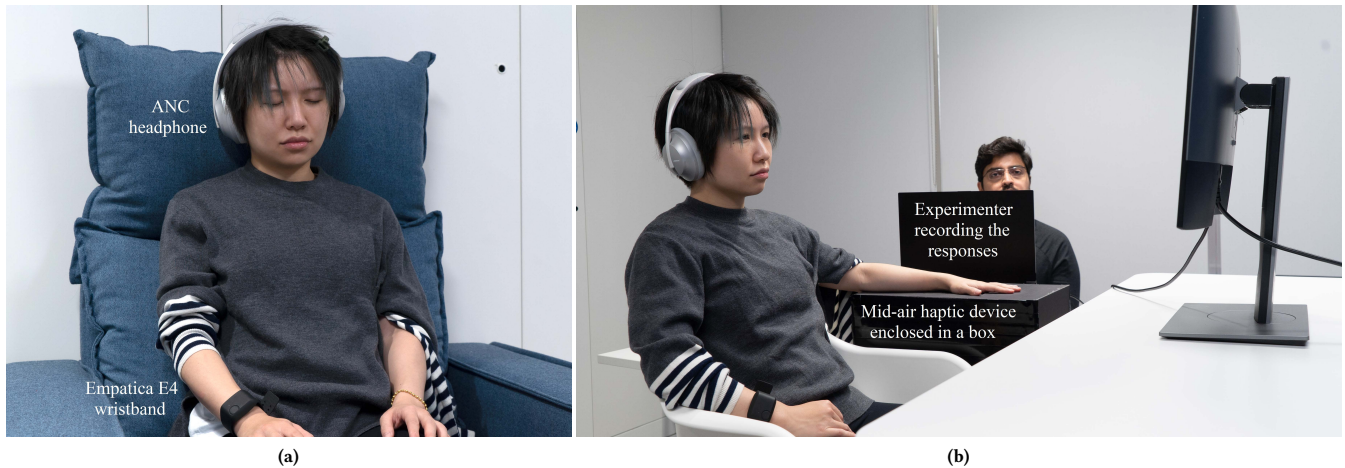
Figure 3: User study setup includes a mid-air haptic device placed inside the black box and a monitor. Participants placed their left arm over the box' aperture (9x10cm) to perceive the stimuli and were wearing the Empatica E4 band on their right wrist to measure their heart rate. (Figure represents the illustration of the user study and not the actual participants.)
