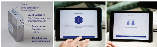
Figure 2: Left: Illustration of the OWidgets scent delivery device prototype, Middle: App interface to dispense the smell for an interactive smell training session. Right: Illustration of an example performance result available to participants at the end of smell training session. Photo Credit: OWidgets Ltd.
