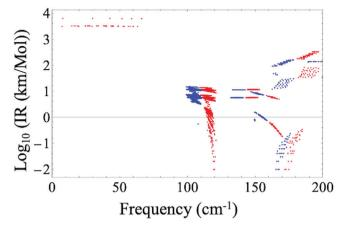
**Figure 3.** A comparison between the computed lowest 15 TO phonon modes for the lattice shrinkage (red) and expansion (blue) for the IR intensities as a function of phonon frequencies. We can clearly see there are many low-frequency phonon mode (softening) for the shrunk lattice. Notice that the Log<sub>10</sub> (IR intensities) are plotted to show a clear contrast between different vibrational modes.
