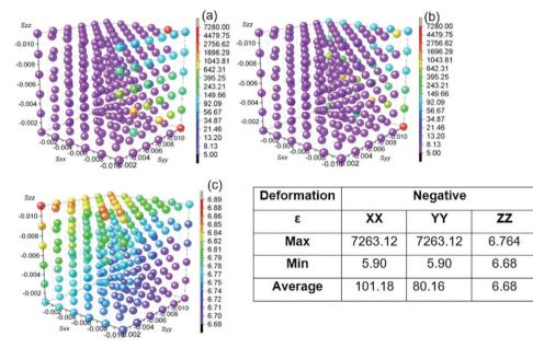
**Figure 2.** The diagonal terms  $\varepsilon_0^{XX}$  a),  $\varepsilon_0^{YY}$  b), and  $\varepsilon_0^{zz}$  c) of the static dielectric tensor as a function of strain (all negative, lattice shrinkage down to -0.011% or -1.1%). The computed dielectric tensor diagonal terms can go up to 7263.12. In the inset table, we have also shown the maximum, minimum, and average values. We can clearly see the significant effects of the strains on the  $\varepsilon_0^{XX}$  and  $\varepsilon_0^{YY}$ .
