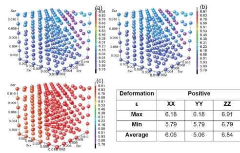
**Figure 1.** The diagonal terms  $\varepsilon_0^{XX}$  a),  $\varepsilon_0^{YY}$  b), and  $\varepsilon_0^{ZZ}$  c) of the static dielectric tensor as a function of strain tensor element  $s_{xx}$ ,  $s_{yy}$ , and  $s_{zz}$  (all positive, lattice expansion up to 0.011% or 1.1%). All the values can only go up to  $\approx 6$ . In the inset table, we also show the maximum, minimum, and average values for the static dielectric tensors.
