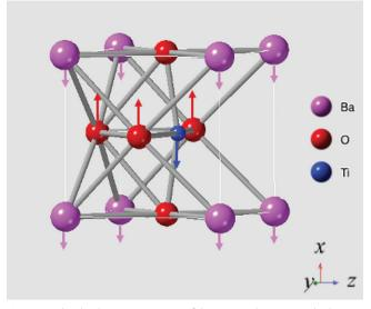
**Figure 5.** The displacement pattern of the ions and anions in the lowest-frequency mode for the calculation with the largest dielectric constant 7263.12 is shown. Ti and Ba (-x) move in the opposite direction as the O atoms (+x), thus enhancing the electrical dipoles and the dielectric constant.
