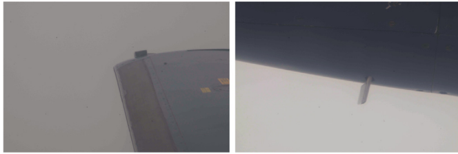
(a) icing on the wing (b) icing on the tube
