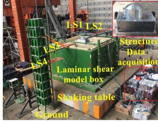
(b) Figure 3 Scaled model and sensor locations: (a) The schematic diagram of the test; (b) photograph of the test.
