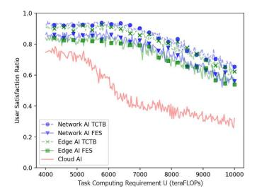
(b) Impact of Task Computing Requirement when Task Density  $\lambda$ =1000.
