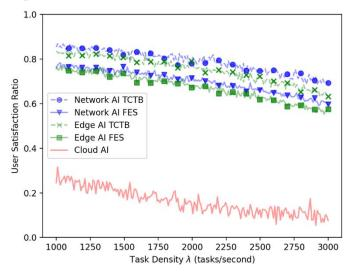
(a) Impact of Task Density when Task Computing Requirement U-N (7 × 10<sup>3</sup>, 10<sup>2</sup>).
