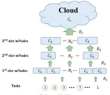
(b) System Model. Fig.2 Three AI Architectures and the System Model.
