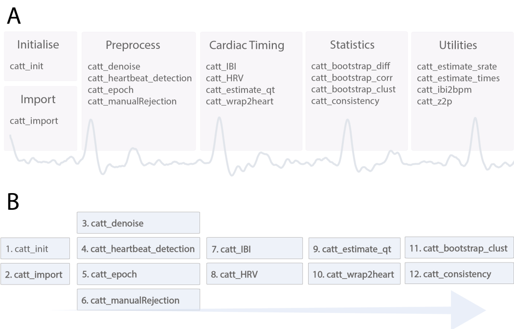
Figure 2. Outline of the CaTT Toolbox. (A) List of Matlab functions included in the toolbox, grouped by their usage. (B) Example flow chart showing the order in which to call the functions. The user needs to begin by initialising the toolbox and calling the data. Next, if they wish to preprocess using CaTT then they would denoise, detect the peaks of the R and T waves, epoch the data into heart beats, then reject epochs with artefacts. Participant-level statistics heart beat variability (HRV) and mean interbeat interval (IBI, in ms) are calculated. Next, the user must estimate the QT interval (according to the method they set in the catt_opts ), onsets are wrapped to the cardiac cycle, and finally, participant- and group-level statistical tests are run.
