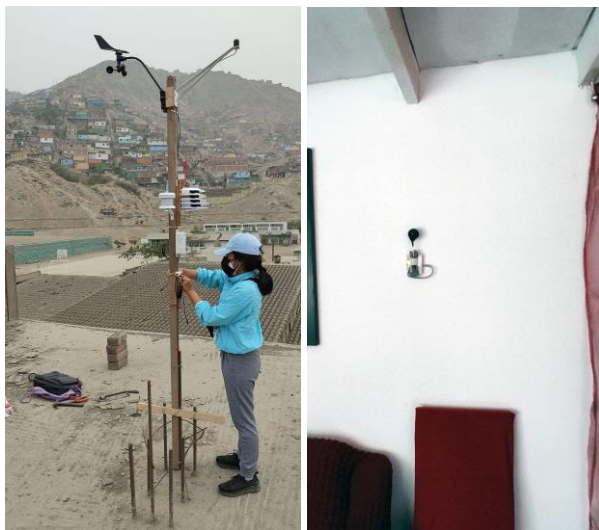
Figure 4. View of the outdoor weather station (left) and data logger inside a house (right).
