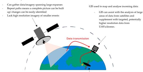
UAVs/Drones can get much closer to the objects it is capturing data from, and have controllable flight paths:
