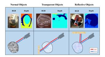
Fig. 2. Depth calculation of different objects.
