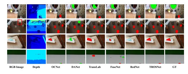
Fig. 13. Visualization of results on TROSD: OCNet [15], DANet [48] and TransLab [8] are RGB based methods; FuseNet [52], RedNet [53] and the proposed TROSNet are RGB-D based methods.
