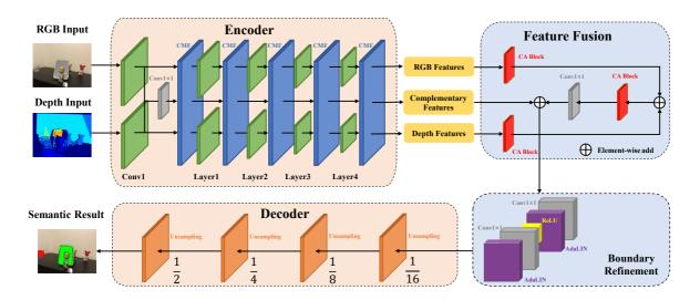
Fig. 9. The overall network structure of TROSNet. Firstly, given an input RGB-D image, we use a two-stream encoder to extract features from RGB and depth images, respectively. Then, we use a Feature Fusion module to fuse RGB and depth features. Next, a Boundary Refinement module is used to refine the boundary details of the features. Finally, a decoder predicts the semantic label maps.
