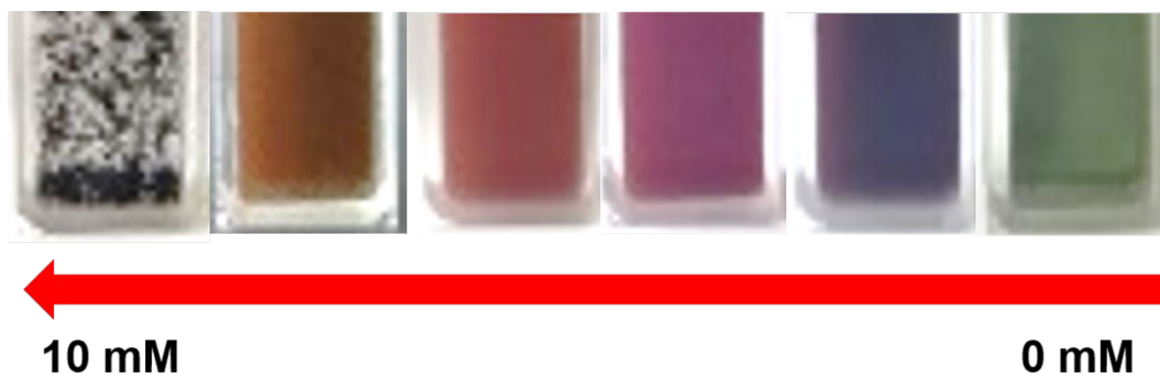
Figure S17. The digital image of \text{Ti}_3\text{C}_2\text{T}_x MXene colloidal suspensions after adding different concentrations of \text{HAuCl}_4 solutions in the range of 0 mM to 10 mM.
