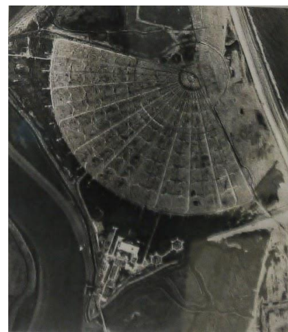
Plan view of the COBRA MIST array, pointing to the North-East. The radius of the fan-shaped array is some 550 m.
