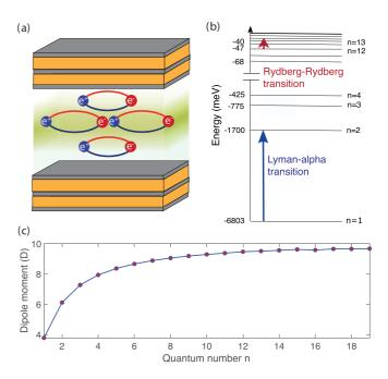
FIG. 1. (a) Sketch of the Ps CQED system, representing Ps atoms interacting with the electromagnetic field trapped in a cavity formed by two DBRs. (b) Energy levels of Ps with the Lyman- $\alpha$  and Rydberg-Rydberg transitions explicitly considered in this paper highlighted (not to scale). (c) Dipole moment  $d_{n \to n+1}$  in debyes as a function of the principal quantum number *n* of the initial energy state.
