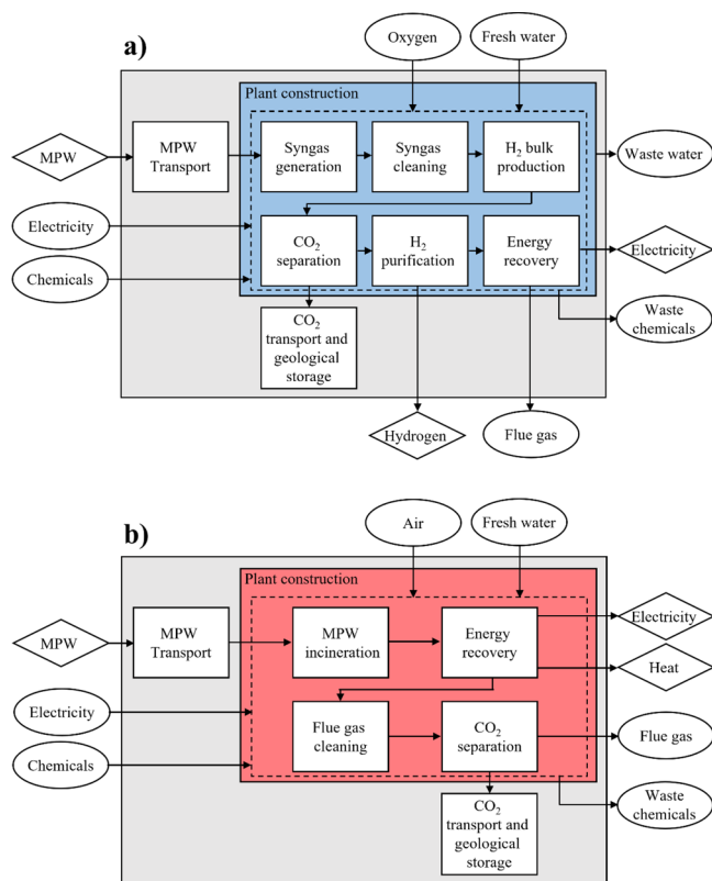
Figure 4. System boundary for the (a) H 2 w/CCS and (b) WtE w/CCS plants.
