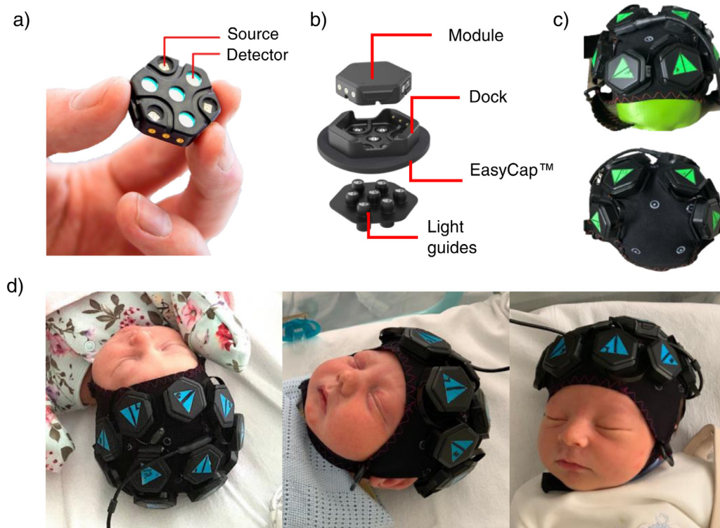
Fig. 3. (a) LUMO tile with source and detector positions indicated. (b) Positioning of docks into which the hexagonal tiles are located. The light-guide piece contains seven short optical fibres with length 4.5 mm. (c) Custom-designed neonatal HD-DOT cap containing 12 LUMO tiles. The 12 tiles and dock chain are integrated into an EasyCap™. Front and back views of the cap are shown. (d) Photographs of the cap on three newborn infants during cot-side data recording with tiles visible over the frontal and parietal cortices.
