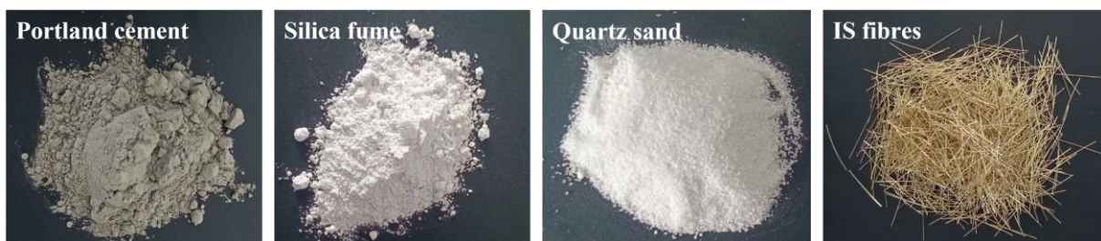
Fig. 2. Photos of Portland cement, silica fume, quartz sand and industrial steel (IS) fibres.
