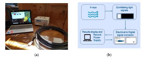
**Figure 1.** (a) DoseVue system: (a.1) DoseWire detector, (a.2) optical fibre, (a.3) extension cable, (a.4) signal convertor interface, (a.5) DoseVue software. (b) Signal acquisition workflow.
