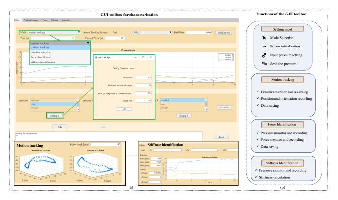
Fig. 6. The design of the GUI toolbox for robot characterisations. (a) Snapshots of the main page for setting, with the motion recording and stiffness identification examples shown at the bottom. (b) The architecture of the GUI. The source codes for the GUI can be downloaded from the GitHub repository.
