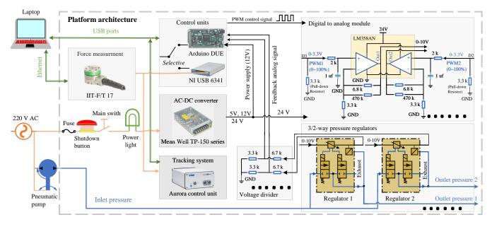
Fig. 5. Connection architecture of the platform. AC power and inlet pressure are provided from external supplies. Data transmission between the laptop and the platform is achieved via USB and Ethernet. Both the Arduino Due and USB-6341 can be selected as the control unit, depending on specific applications.
