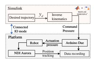
Fig. 9. Control scheme of implementing the inverse kinematics to the platform using Simulink.
