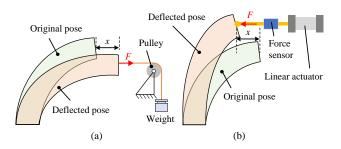
Fig. 2. Stiffness measurement demonstrated on a soft robotic manipulator applying (a) a pulling and (b) a pushing force. The force F results in a displacement or deflection x along the force direction.
