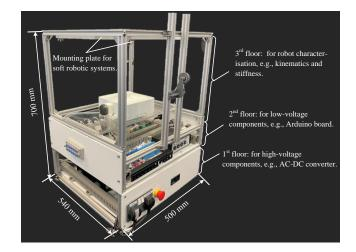
Fig. 1. Physical platform for actuation, characterisation (e.g., kinematics, stiffness and force identification), control implementation and validation of pneumatically driven soft robotic system. The platform consists of three floors covering high-voltage components, DC components and characterisation space. The CAD drawing in Fig. 4 gives a detailed view.
