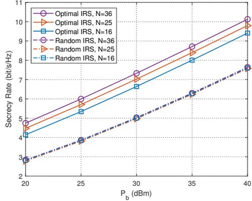
Fig. 4. Secrecy performance comparison between the optimal IRS scheme and the random IRS benchmark with different  $P_b$  and  $N$ .
