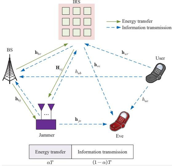
Fig. 1. Uplink system model with the help of IRS and jammer.
