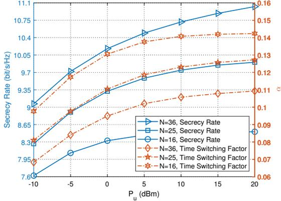
Fig. 3. Performance comparison of secrecy rate and time switching factor  $\alpha$  with different user transmit power.  $N = 16, 25$  and  $36$ .
