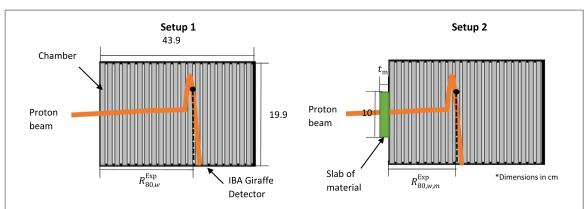
**Figure 1.** Experimental setup for water-equivalent thickness measurements (without - setup 1, left - and with - setup 2, right – phantom material in front of the Giraffe detector). The number of ionization chambers shown within detector is reduced to simplify the schematic.
