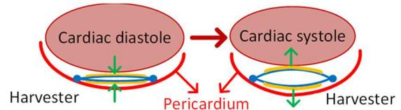
Fig.1 Piezoelectric energy harvester placement in the heart.
