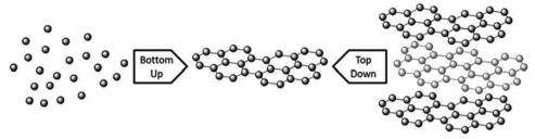
Figure 4. Illustration of top-down and bottom-up synthesis methods of graphene. Reproduced (Adapted) with permission. [22] Copyright 2013, RSC.
