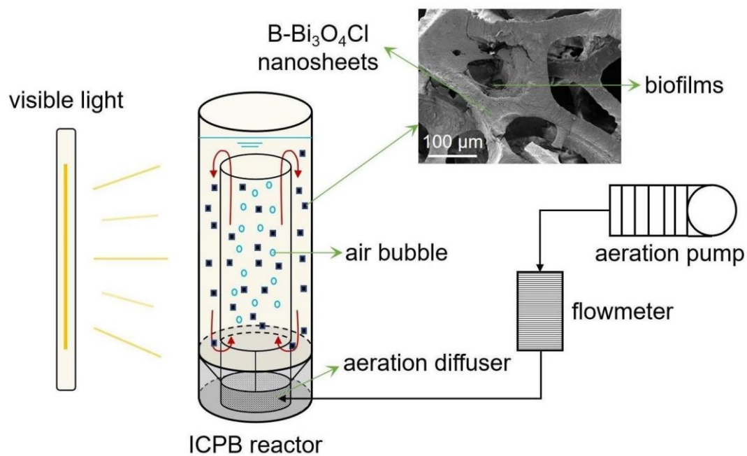
994 Fig. S4. Schematic diagram of the photocatalytic circulating-bed biofilm reactor.
