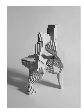
Figure 1. Chair 'Model T1-M', after 860 generations (86,000 structural evaluations)
