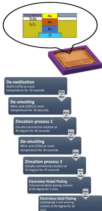
Fig. 3. Diagram of a Au coated pad on a CMOS chip. Schematic shows the steps of Au electroless deposition process via zinc/nickel route [46].
