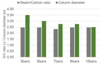
Fig. 12. DISPLACE steam demand and column diameter for different operating pressures at similar CO2 purity and capture ratio.
