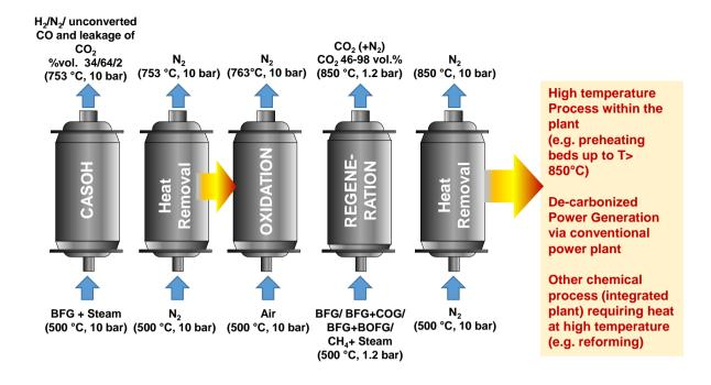
Fig. 6. CASOH scheme reaction network using BFG for both  $H_2/N_2$  production and sorbent regeneration (other low  $N_2$  content fuel gases such as NG, BOFG and COG can be used in the regeneration stage to further increase purity of CO<sub>2</sub>).
