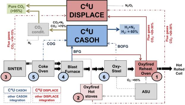
Fig. 9. Block flow diagram of main production units in a steel mill integrated with C<sup>4</sup>U CO<sub>2</sub> capture technologies.
