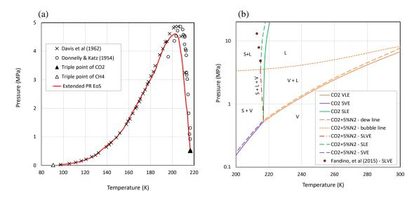
Fig. 15. P-T phase diagrams for CO<sub>2</sub> binary mixtures with impurities [31]: (a) Solid-Liquid-Vapour Equilibria (SLVE) locus for CO<sub>2</sub> + CH<sub>4</sub> system; (b) impact of CO<sub>2</sub> dilution by 5% N<sub>2</sub> on the predicted phase transition boundaries (V – vapour, L – liquid, S - solid).
