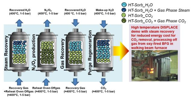
Fig. 2. The general process sequence of stages for the DISPLACE process applied to off-gases from reheating furnaces.
