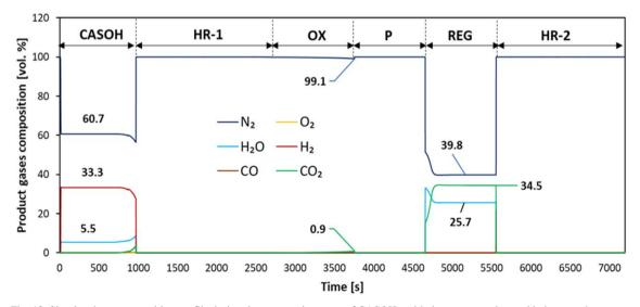
Fig. 13. Simulated gas composition profile during the consecutive stage of CASOH, oxidation, regeneration and in between heat removal [23].
