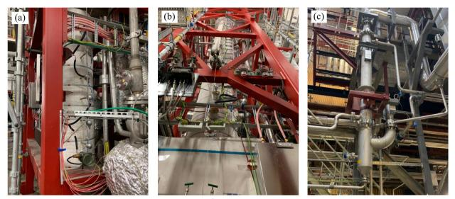
Fig. 5. DISPLACE CO<sub>2</sub> capture equipment: (a) WGS reactor for C<sup>4</sup>U-SEWGS campaign; (b) single column DISPLACE capture unit; (c) syngas cooler.
