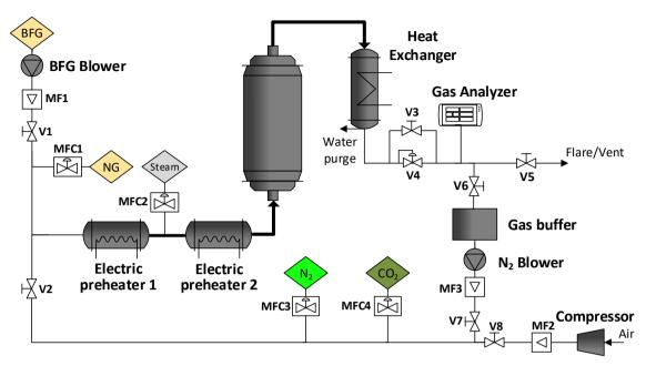
Fig. 7. Simplified process flow diagram of the CASOH pilot.
