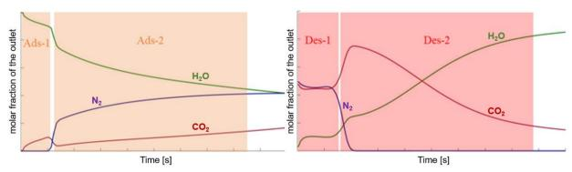
Fig. 10. Representative examples of the DISPLACE column outlet profiles for adsorption (left) and desorption (right).
