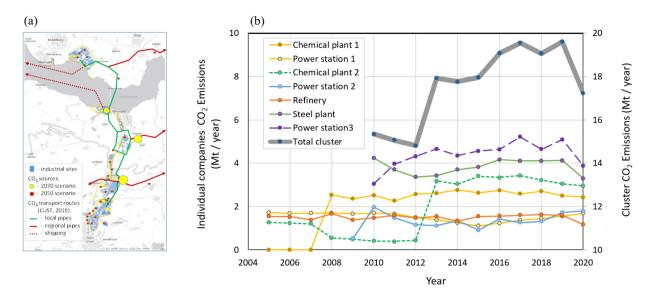
Fig. 16. Characterisation of the North Sea Port industrial cluster: (a) map showing locations of CO<sub>2</sub> emission sources and transport routes by pipeline and shipping [33]; (b) historical CO<sub>2</sub> emission rates for individual emitters and total industrial cluster.
