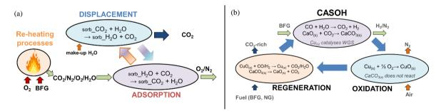
Fig. 1. Conceptual representation of two examples of application of the C<sup>4</sup>U high temperature solid looping technologies for steel mills: (a) DISPLACE; (b) CASOH.
