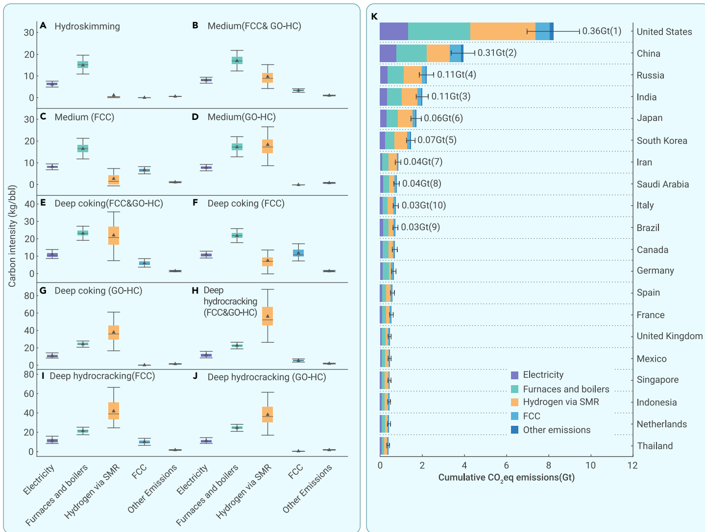
Figure 3. GHG emissions based on process units GHG emissions based on process units in (A) hydroskimming refineries, (B) medium conversion refineries (FCC), (C) medium conversion refineries (GO-HC), (D) medium conversion refineries (FCC&GO-HC), (E) Deep coking refineries (FCC), (F) deep coking refineries (GO-HC), (G) deep coking refineries (FCC&GO-HC), (H) deep hydrocracking refineries (FCC), (I) deep hydrocracking refineries (GO-HC), and (J) deep hydrocracking refineries (FCC&GO-HC). (K) Cumulative GHG emissions based on process units in the top 20 countries. The number in Figure 2K represents GHG emissions from the refining industry in the top 20 countries in 2021.
