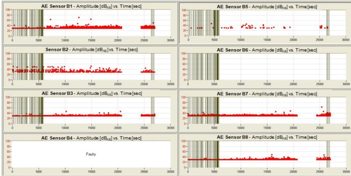
Figure 15: AE recording during 8-h monitoring under normal traffic: amplitude vs. time (screen shot of the acquisition software) [63].
