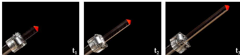
Fig. 8. The torsional actuator, based on the development of a configuration force, transforms a twist into a longitudinal thrust through a release of the elastic energy, without any use of gears or other transmission mechanisms.
