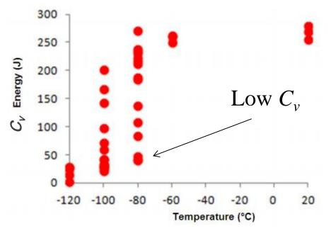
Charpy impact test energy for X70 grade steel
