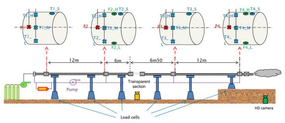
Schematic representation of the test pipeline (40 m long, 50mm i.d.), showing the ethylene feeding equipment, and the locations of the pressure, temperature and heat flux transducers along the pipe.
