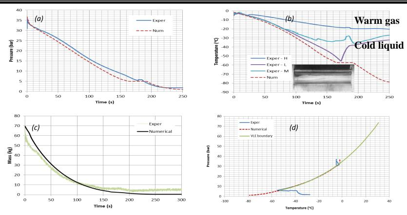
The history of variation of the fluid pressure (*a*), temperature (*b*) and the pipeline inventory (*c*) as predicted by the flow model in comparison with the CO2QUEST data (INERIS puncture Test 14). (*d*) - pressure-temperature diagram showing the CO<sub>2</sub> vapor saturation line and the pipeline decompression trajectory
