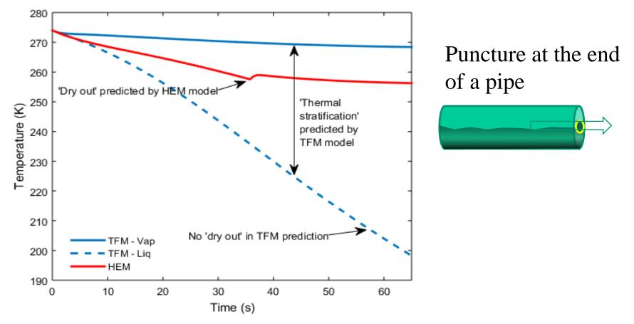
History of the fluid temperature variation in the pipeline near the rupture location. Predictions by HEM and TFM models. Pipe length 37m, pipe i.d. 50 mm, puncture diameter 12mm. Initially the fluid is saturated 50% v/v liquid at  $0^{\circ}$ C.
