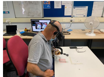
Figure 1 - Participant using the system. Showing the HapticMASTER robot, Oculus Rift and experimenter's screen.
